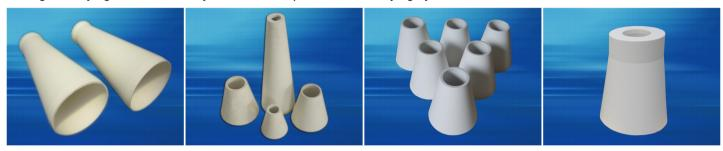
When cyclone is at work, the rotary motion of material generates great centrifugal force, the inwall of cyclone is worn at high speed. For dense material, the abrasion of inner is extremely worse under high impact by centrifugal force. One-piece alumina ceramic tube is used as wear resistant lining in cyclone by its high hardness, strength, abrasion resistance and economic practicality.
